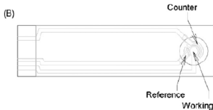
Fig. 3. (A) Antiport transport cycle for a printed DO sensor. (B) Layout of the electrodes on the substrate (overall dimensions: 20 mm × 70 mm; working electrode: 4 mm diameter; membrane opening in the covering dielectric: 13 mm diameter).
